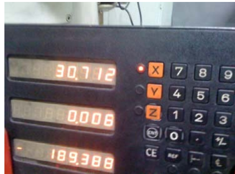
Figure 5. Values measured with the interferometer Figure.6 Values shown on the machine's display
