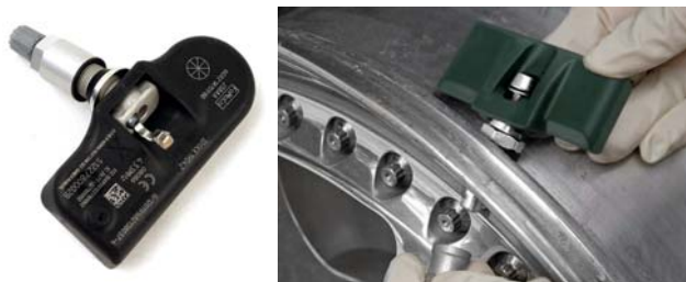
Figure 2. Sensor of direct TPMS system
