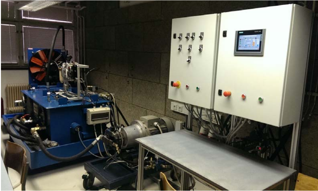
Figure 2. Supply and control system with a 2x15 kW power train
