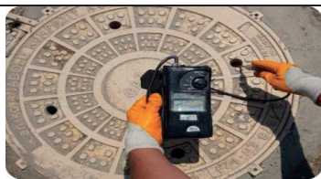
Figure 4. Manhole Cover Leakage Test
