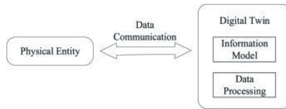
Figure 1. General reference model of digital twin [2]
